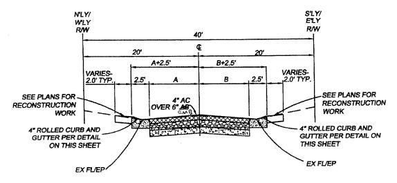
REMOVE EXISTING ± 4" AC PAVEMENT AND ± 6" BASE/SAND
