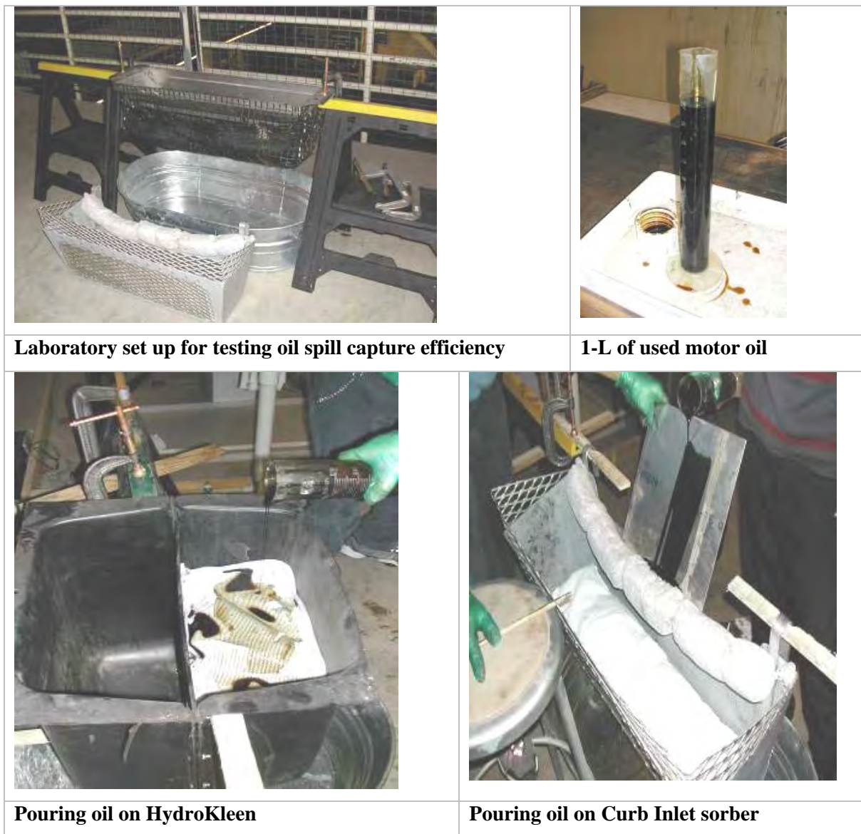
Figure 4-21: Laboratory set up for the evaluation of spill control by catch basin inserts.
