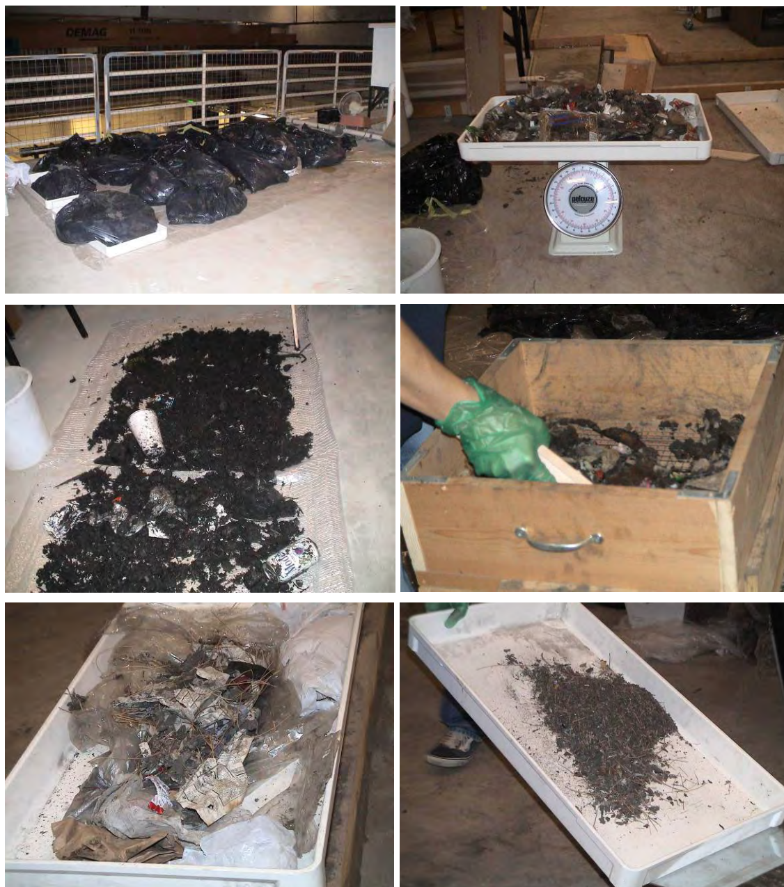
Figure 4-26. Photos of bulk solids screening process.
