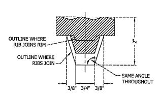
CROSS SECTION THRU RIB AT MID RADIUS
