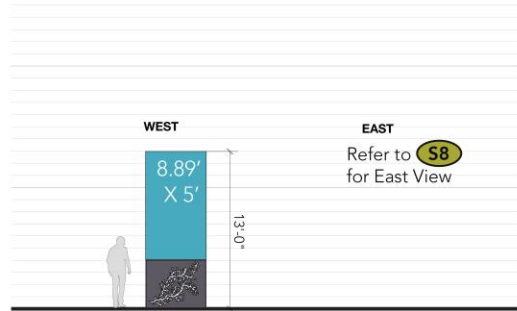
D1 FREESTANDING DISPLAY AT CENTRAL PLAZA EAST NEAR CEDAR WAY LED 4 MM OUTDOOR
