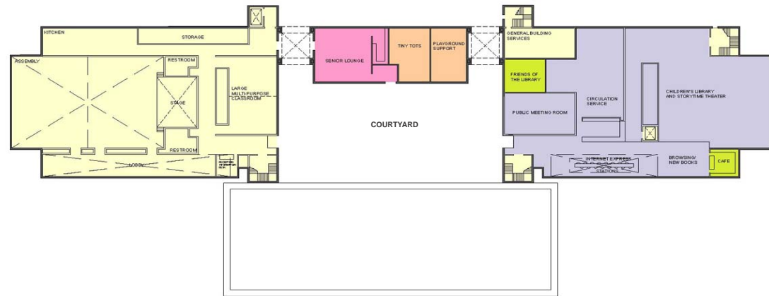
Facilities Recommended for Live Oak Park Illustrative First Floor Plan. The friends of the library, cafe and coffee shop, public meeting room, circulation services and children’s library of the library, the main hall, kitchen and meeting rooms of the community center the lounge and kitchen of the senior center and the tot lot and children’s playground program share the ground floor in this illustration of facilities recommended for Live Oak park.
