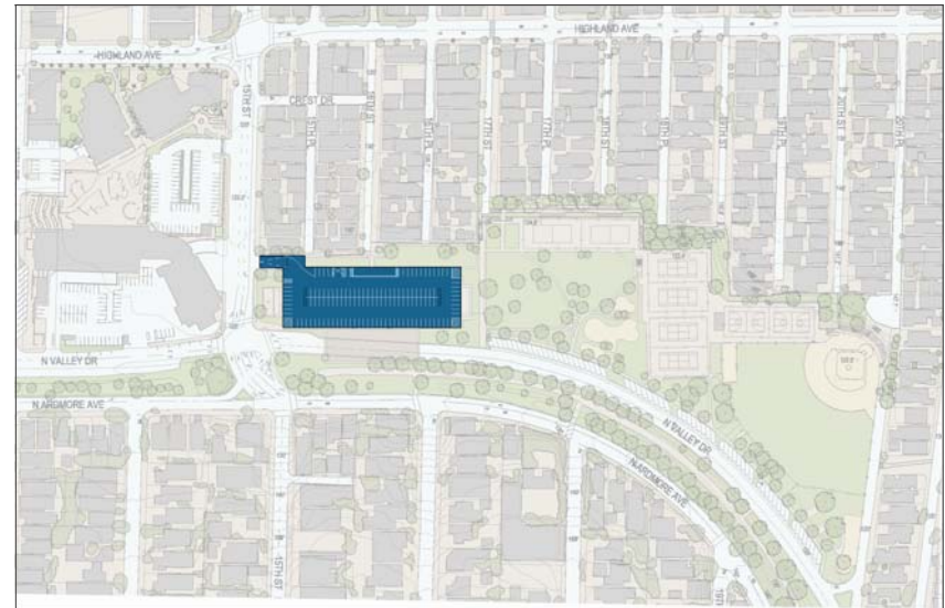
Live Oak Park Below Grade Parking in the Illustrative Plan. One hundred and thirty spaces are provided in a single level beneath the library and community center. The structure is accessed via a ramp at 15th street.
