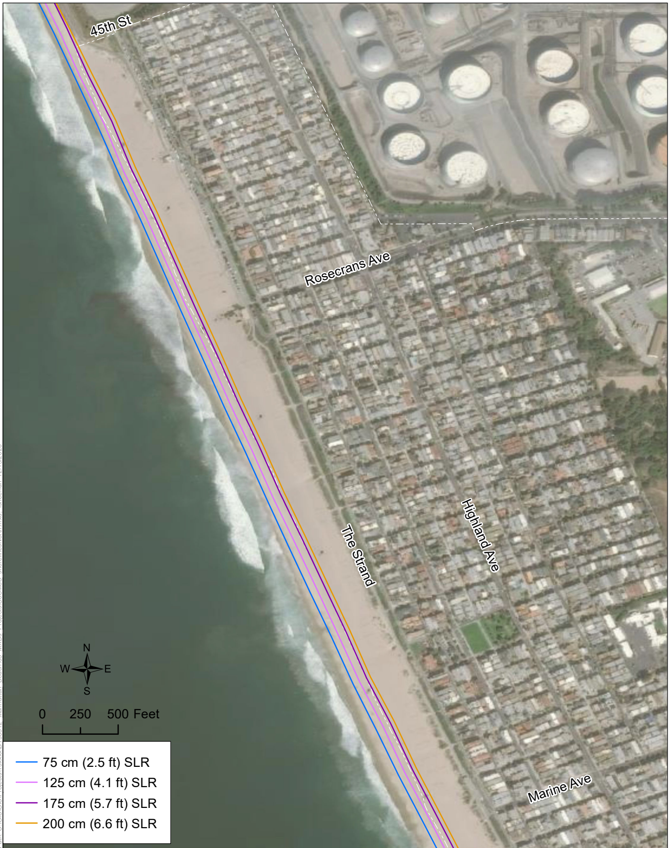
Figure 3-9 Shoreline Erosion with Sea Level Rise in North Manhattan Beach
