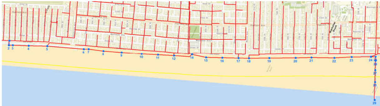
Figure 2. Map of sewer pipe segment endpoints extracted from City shapefiles.
