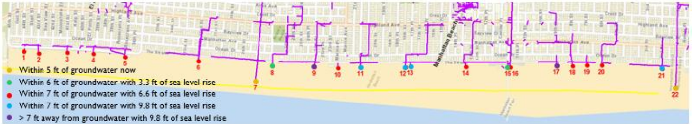
Figure 4-2: Stormwater Outfall Locations
