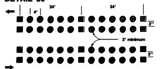
Alternate to Detail 29. For use at problem locations where it is difficult to place and maintain lines because of moisture, sand, etc.
