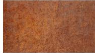
CORTEN STEEL 1/4" PLATE SAMPLE
