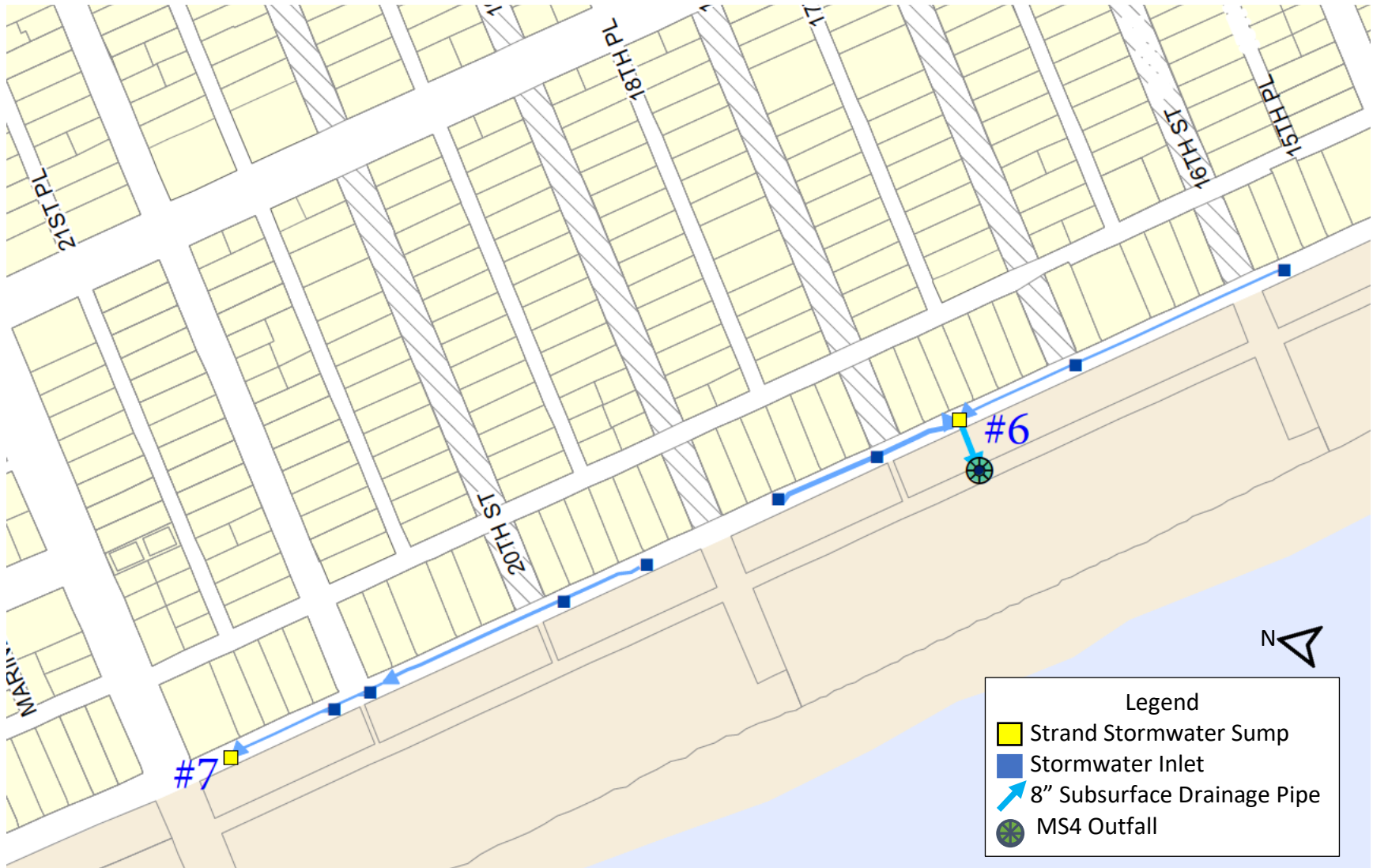
Map 3 Strand Drainage System Configuration: Collection Basin #6 and Sump #7
