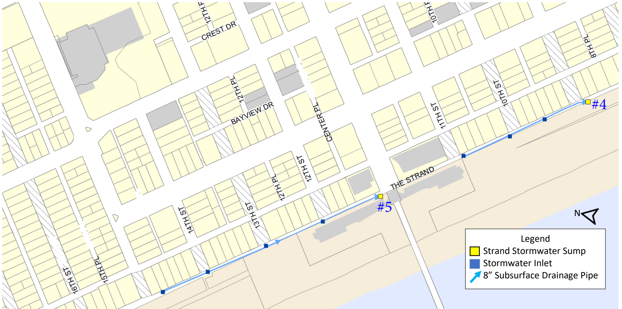
Map 2 Strand Drainage System Configuration: Sumps #4-5
