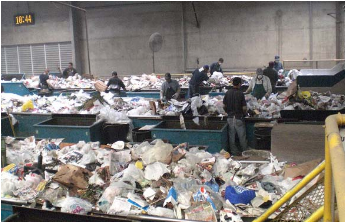
Figure 7 -- Typical Waste Stream Traveling Along a Conveyor Belt
