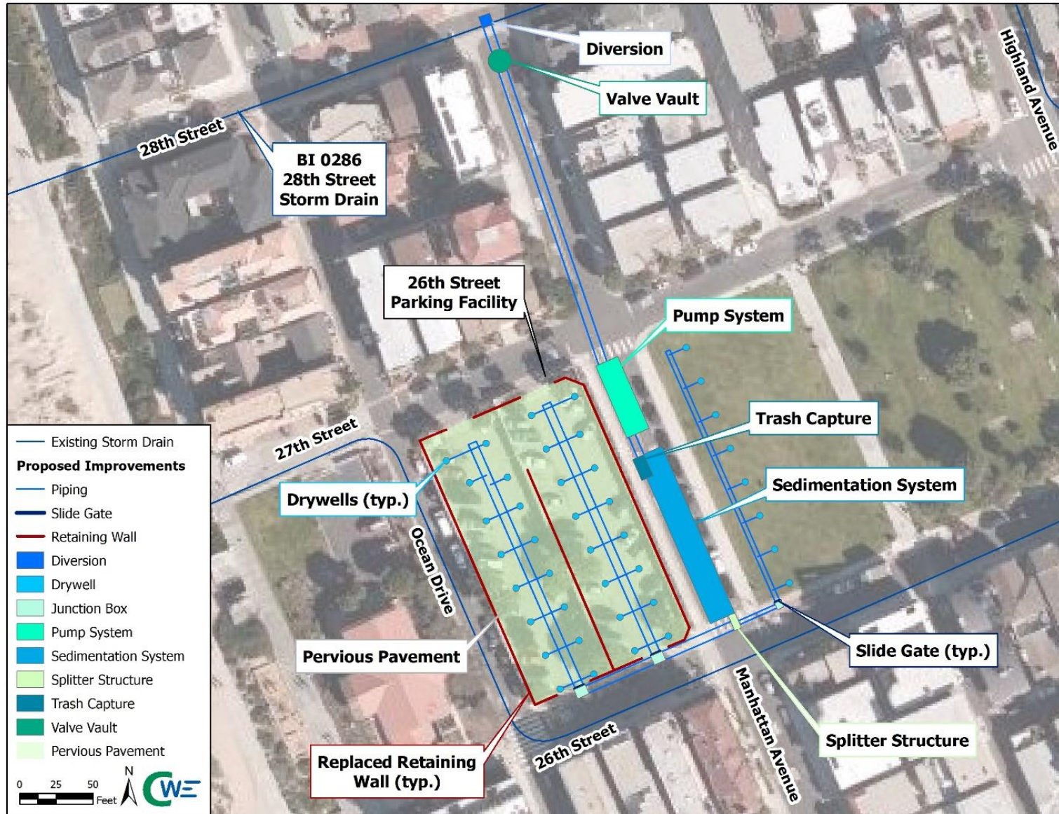
Figure 2 Stormwater Infiltration Concept
