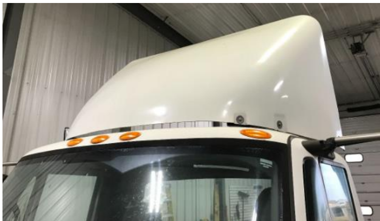
Example of wind-fairing equipment on top of a cab.
