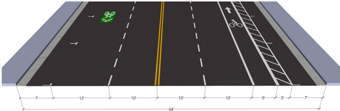
Figure 19 Cross section 64-6a – Shared lane markings downhill, buffered bike lane uphill, 4 lanes
